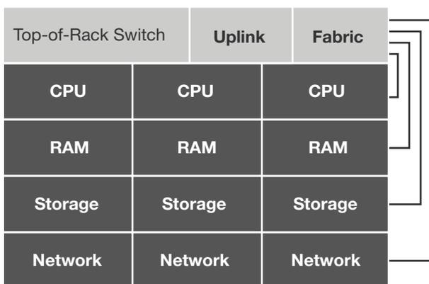
**Figure 11-3:** Disaggregated resources at the rack scale
