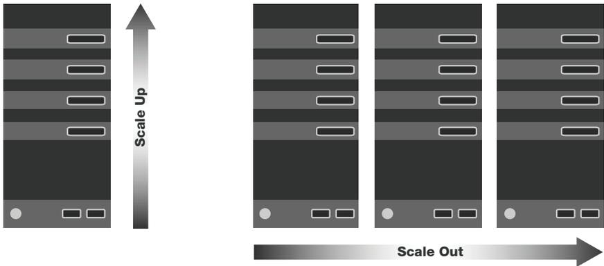
**Figure 8-3:** Scale Up vs. Scale Out Architecture
