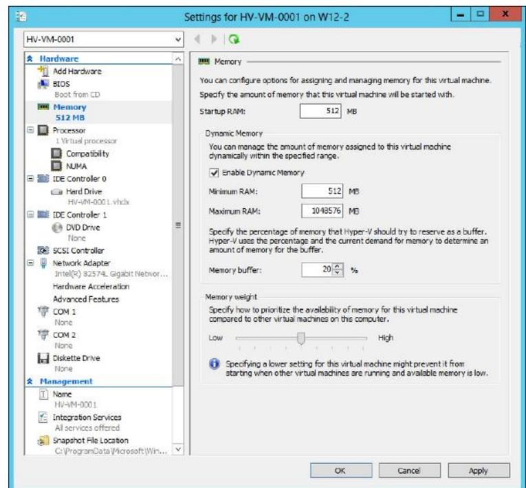
It's easy to see how this feature could reduce a virtual machine's memory to dangerous levels, leaving it unable to respond to a sudden environmental change that creates the need for more memory. To prevent this situation, Hyper-V provides a (default) buffer of 20% of unused memory.
