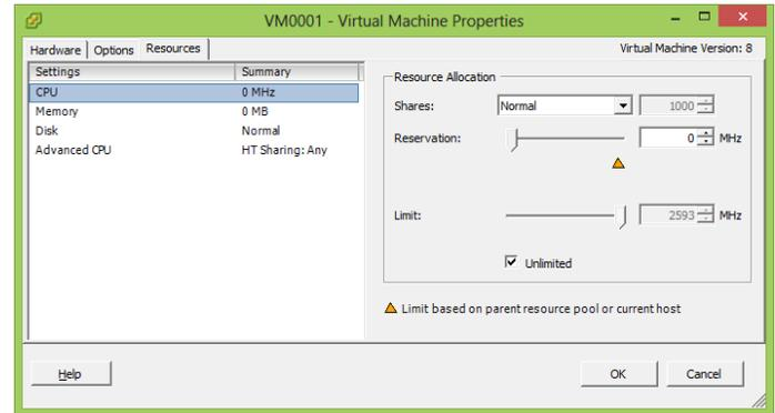
At the host level, vSphere has a powerful CPU scheduling mechanism in place that ensures that virtual machines receive attention from the system. VMware has produced a [white paper](#) that goes into great technical depth for how this scheduling is achieved.
