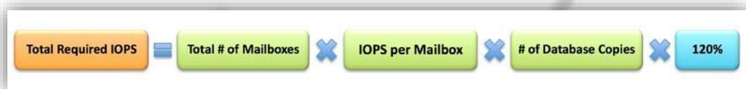
FIGURE 3: EXCHANGE IOPS CALCULATION FORMULA
