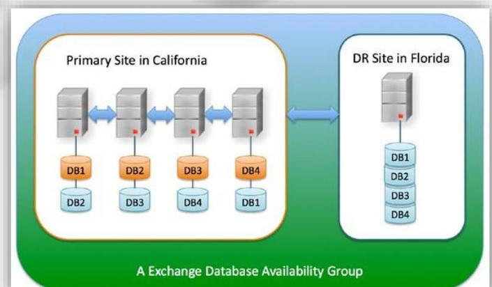
FIGURE 4: EXCHANGE 2010 DAGS IN ACTION
